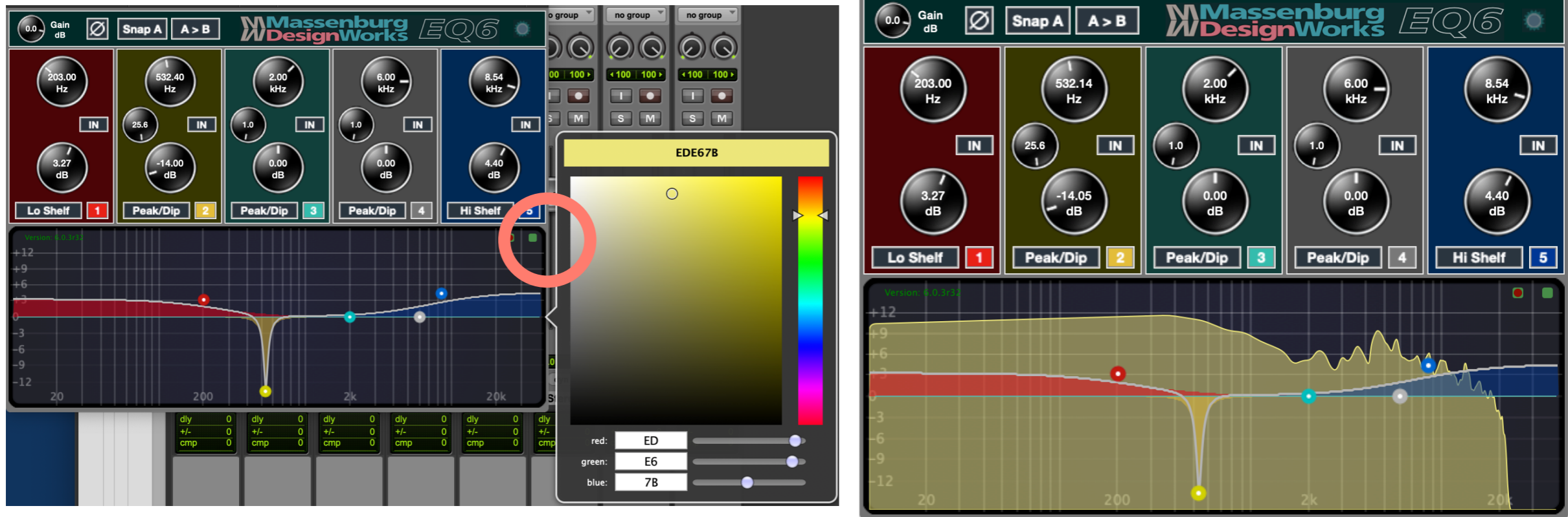
Figure above left - ToolTip in the upper corner. Right - Color change made is reflected
