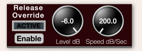
The **Level** control indicates the number of decibels a signal must change relative to the speed of the two primary **Timing** controls in order to override their settings. Turning clockwise, the release override will occur more frequently. Turning counter-clockwise, more precipitous changes in level are required, and/or slower Timing settings.
