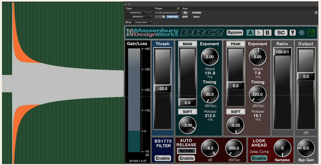
Finally, to soften the transition between **MAIN** control and **PEAK** control, you could increase the **Soft Knee** of the **PEAK** section (shown in blue).
