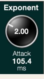
Unlike its GML8900 predecessor, **MDWDRC2** exposes the mathematical aspect of the **Timing** controls to user input via the **Exponent** control. The decimal values themselves are quite literally the exponents used in the math to determine a range of detection, from average to True RMS, to degrees of peak loudness in a musically useful way. A more technical explanation can be found in the <u>Appendix</u>.
