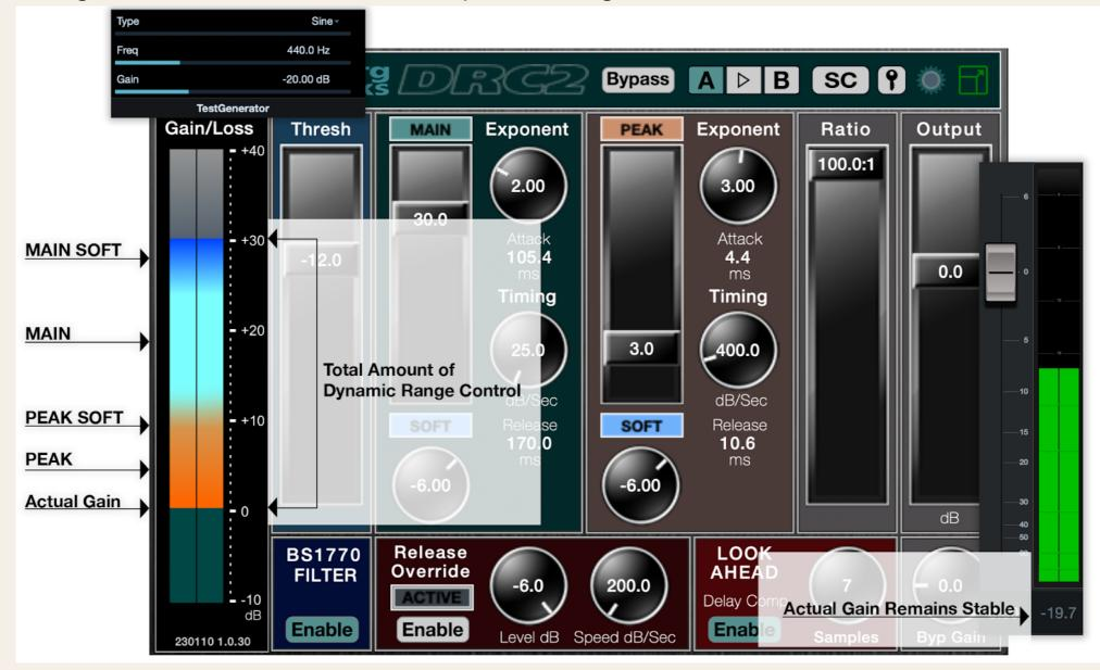
**Dark Green / Dark Gray** The *gain/loss* of the plugin is indicated by the division between the top of the dark green and the bottom of the dark gray, and always represents the instantaneous *static* gain of the plugin. *If there are no other colors, there is no automatic gain control active.*
